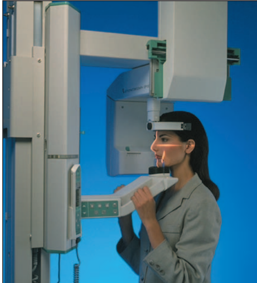
Figure 11 Positioning guides; note the bite rod, head guides, and aiming light
